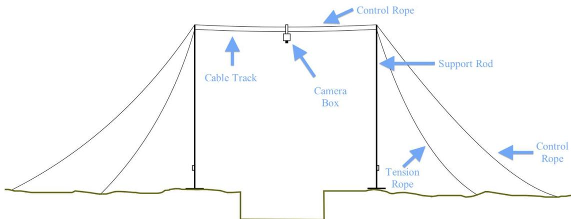
**Figure 2: Schematic of the Karsola Overhead Photography System**
