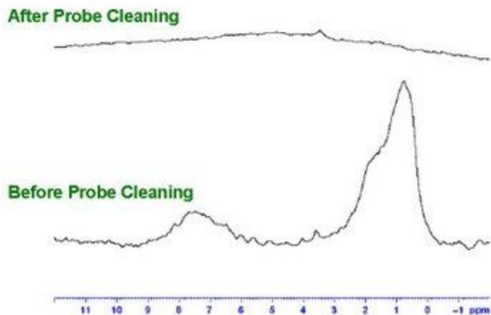
1 H NMR Spectra of an Empty 5 mm Tube in an NMR Probe Before and After the Probe Was Cleaned
