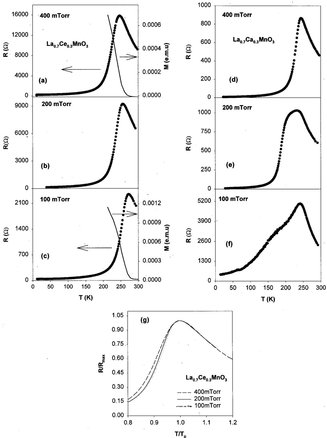
FIG. 3. Resistance vs temperature of  $La_{0.7}Ce_{0.3}MnO_3$  grown at (a) 400 mTorr, (b) 200 mTorr, (c) 100 mTorr. Resistance vs temperature of  $La_{0.7}Ca_{0.3}MnO_3$  grown at (d) 400 mTorr, (e) 200 mTorr, (f) 100 mTorr; (g) shows the  $R/R_{max}$  vs  $T/T_p$  for the three  $La_{0.7}Ce_{0.3}MnO_3$  films, where  $R_{max}$  is the resistance value at  $T_p$ .
