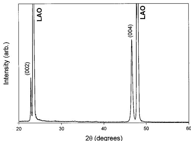
FIG. 1. X-ray  $\theta$ - $2\theta$  scan of the  $\text{La}_{0.7}\text{Ce}_{0.3}\text{MnO}_3$  film grown at 400 mTorr showing the (00 $\ell$ ) peaks of the orthorhombic structure. The peaks marked LAO are the  $\text{LaAlO}_3$  substrate peaks.
