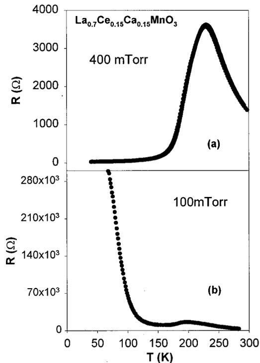
FIG. 4. Resistance vs temperature for  $\text{La}_{0.7}\text{Ca}_{0.3}\text{Ce}_{0.15}\text{MnO}_3$  films grown at (a) 400 mTorr and (b) 100 mTorr oxygen pressure.
