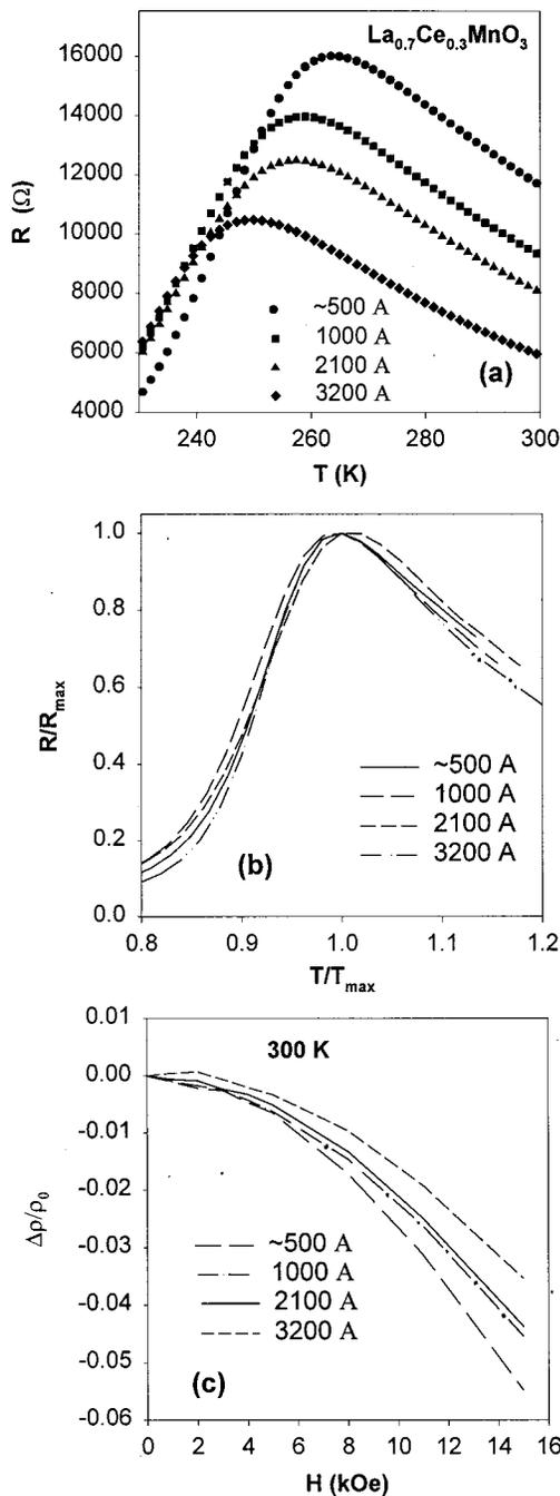
FIG. 6. (a) Resistance vs temperature around  $T_p$  for films of various thickness; (b)  $R/R_{max}$  vs  $T/T_p$  for films of various thickness; (c) MR vs field at 300 K for films of various thickness.
