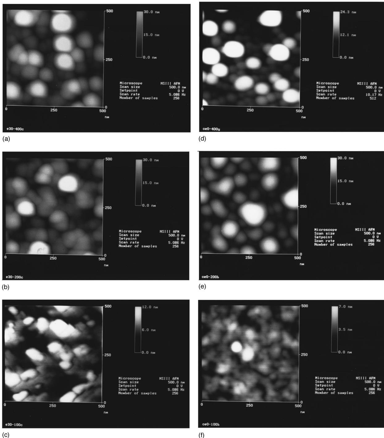
FIG. 2. AFM photograph of the  $\text{La}_{0.7}\text{Ce}_{0.3}\text{MnO}_3$  films grown at (a) 400 mTorr, (b) 200 mTorr, (c) 100 mTorr. AFM photograph of the  $\text{La}_{0.7}\text{Ca}_{0.3}\text{MnO}_3$  films grown at (d) 400 mTorr, (e) 200 mTorr, (f) 100 mTorr.
