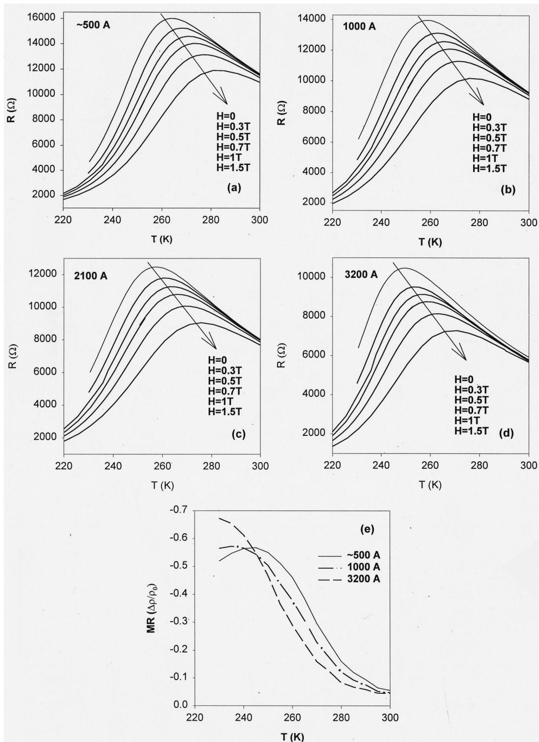
FIG. 7. (a)–(d) Resistance vs temperature at different fields for various film thickness. (e) MR at 1.5 T as a function of temperature for films of various thickness.
