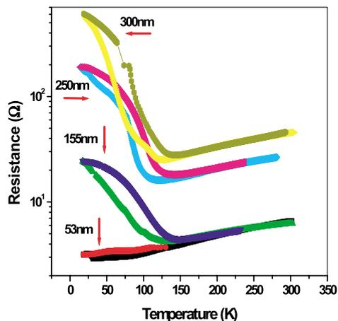
Fig. 7. Resistance versus temperature curves of NdNiO<sub>3</sub> films of various thicknesses grown on LaAlO<sub>3</sub> substrate at 750 °C.
