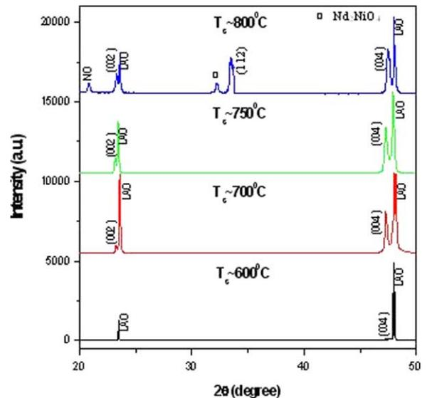
Fig. 2. X-ray diffraction patterns of  $\text{NdNiO}_3$  films grown on  $\text{LaAlO}_3$  substrate at various deposition temperatures.
