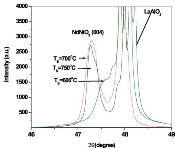
Fig. 3.  $\theta$ – $2\theta$  scans of (004) reflection of NdNiO<sub>3</sub> films deposited at various deposition temperatures.
