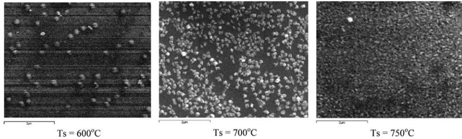
Fig. 4. SEM photographs of NdNiO<sub>3</sub> films deposited on LaAlO<sub>3</sub> substrate at (a) 600 °C (b) 700 and 750 °C.
