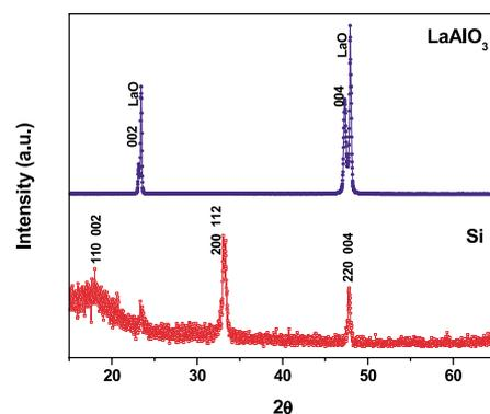
Fig. 6. X ray diffraction patterns of NdNiO<sub>3</sub> films deposited on Si and LaAlO<sub>3</sub> substrate at (a) 675 °C and (b) 750 °C, respectively.
