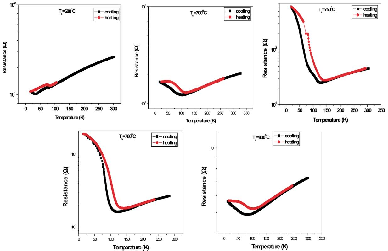
Fig. 1. Resistance versus temperature curves of  $\text{NdNiO}_3$  films deposited on  $\text{LaAlO}_3$  substrate at various deposition temperatures.
