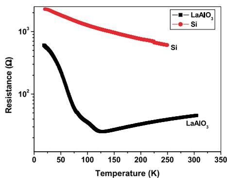
Fig. 5. Resistance versus temperature curves of NdNiO<sub>3</sub> films deposited on Si and LaAlO<sub>3</sub> substrate at  $T_s = 750$  °C.
