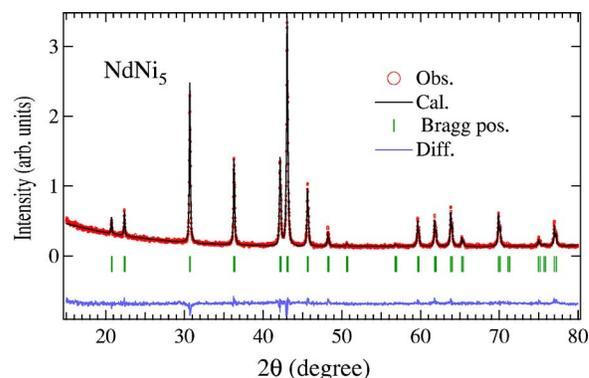
FIG. 1. (Color online) The observed and calculated x-ray-diffraction pattern of NdNi<sub>5</sub> along with their difference. The vertical bars indicate Bragg reflections.
