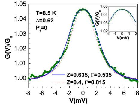
FIG. 4. (Color online) Comparison of the fits of PCAR spectra for Nb-NdNi<sub>5</sub> contact at 8.5 K with two sets of fitting parameters shown in solid and dashed lines. The fit parameters for the two fits are shown in the figure.  $\Delta$  and  $\Gamma$  are in meV. The inset is an enlarged view for the low-bias region.
