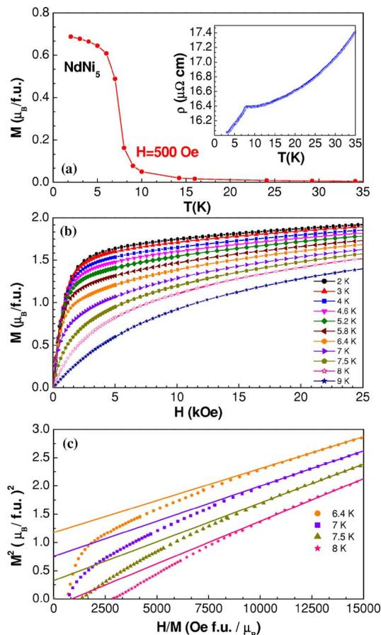
FIG. 2. (Color online) (a) Magnetization vs temperature of NdNi<sub>5</sub> measured in 500 Oe. The inset shows the resistivity as a function of temperature. (b) Isothermal  $M$ - $H$  curves at various temperatures. (c) Arrott plots ( $M^2$  vs  $H/M$ ) at four temperatures close to  $T_C$ .
