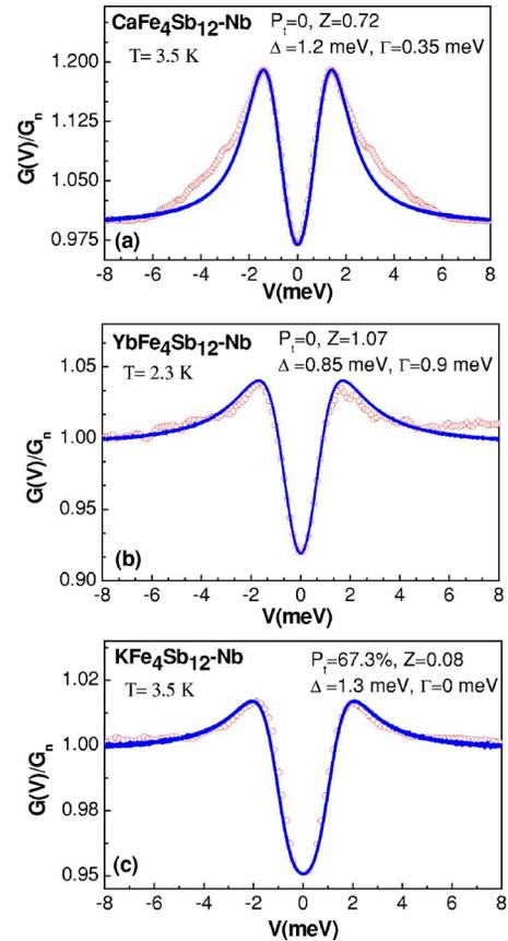
FIG. 6. (Color online) Normalized PCAR spectra for (a) CaFe<sub>4</sub>Sb<sub>12</sub>-Nb point contact at 3.5 K; (b) YbFe<sub>4</sub>Sb<sub>12</sub>-Nb point contact at 2.3 K; (c) KFe<sub>4</sub>Sb<sub>12</sub>-Nb point contact at 3.5 K. The solid lines are the best fits of the spectra to the modified BTK model. The best-fit parameters are also shown in the figures.
