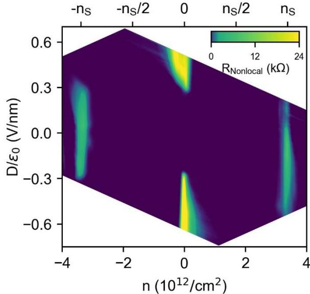
**Caption:** A colour-scale plot of resistance with doping in x-axis and electric field in y-axis. Peaks in the resistance (yellow and green colour) are signatures of valley current.
