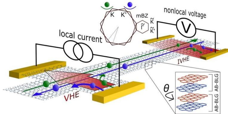
**Caption:** Schematic of the fabricated twisted double bilayer graphene device, along with the valley current flowing through the bulk.
