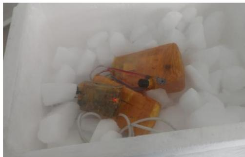
SWAEROSAT-1 payload during low temperature tests in dry ice.
