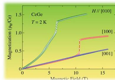
Anisotropic magnetization in CeGe single crystal. The [010] direction represents the easy axis of magnetization
