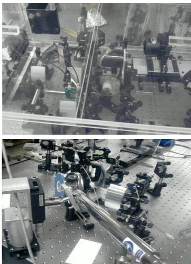
Two home built THz setups for performing transmission (box enclosed) and reflection THz.
