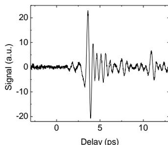
A Typical THz Pulse waveform recorded in our laboratory. The entire pulse duration is in few picoseconds.
