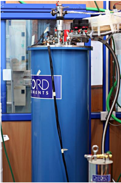
Variable temperature insert for 300mK and 14 T measurements
