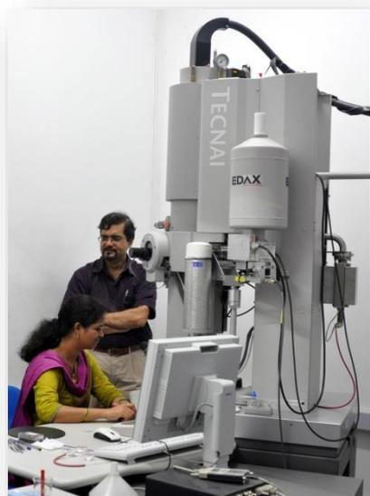
A Transmission Electron Microscope used for imaging nanostructures
