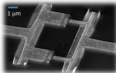
**Top:** Scanning Electron Microscope image of a superconducting qubit.
