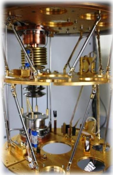
A dilution refrigerator capable of cooling to a temperature of 10 mK
