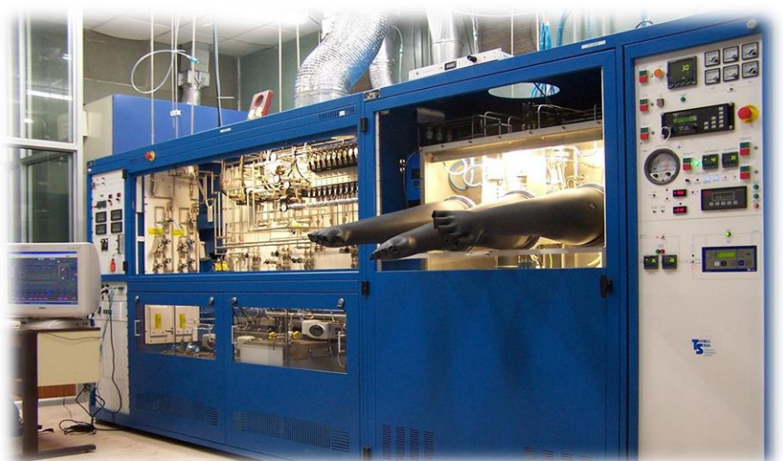
Showerhead MOVPE system for the synthesis of III-nitride materials. The system can handle 3 2-inch wafers, and is equipped with an in-situ real-time optical sensors for measuring surface temperature, growth rate, and sample curvature.
