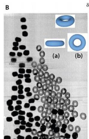
Auto-Partitioning of particles into rolling and sliding states, a mechanism via which friction can be self-adjusted by the system
