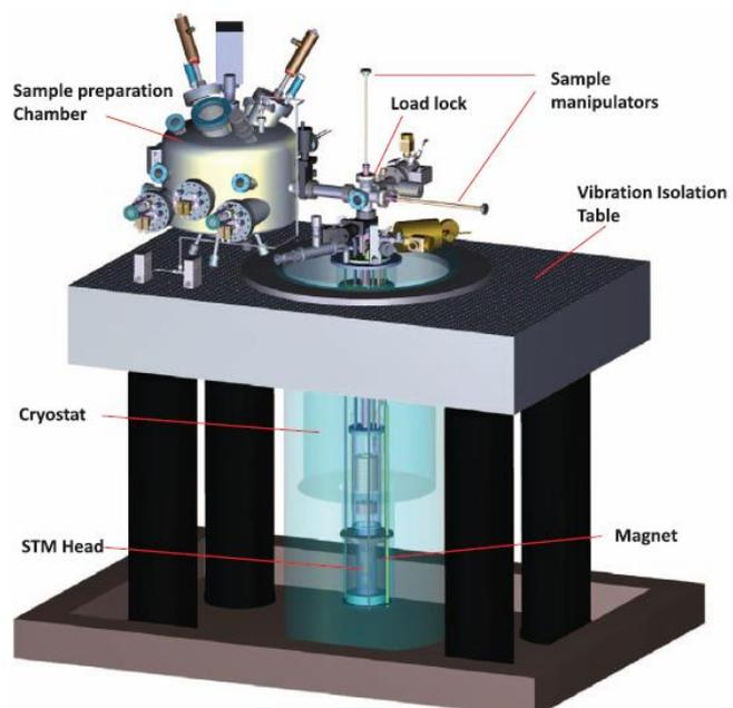
Schematic view of the 350 mK scanning tunneling microscope at TIFR.
