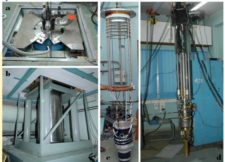
'a' shows the cryostat mounted on active vibration isolation pads.
