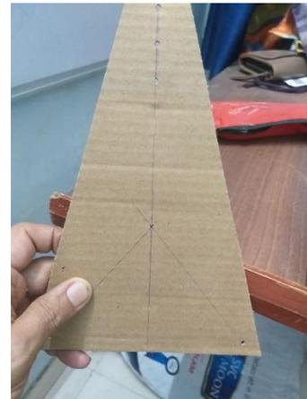
The last picture indicates the centre of mass of the object. Let  $h$  be the length of the triangle from the top most tip to the base and  $b$  be the width of the base. A triangle which oscillates around the axis passing through the tip, moment of inertia can be calculated using the formula
