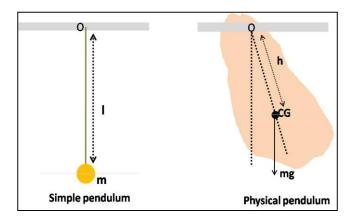
In this experiment we consider a triangular plate of mass m which oscillates in its own plane. Its moment of inertia about an axis passing through its point of suspension O is given by:
