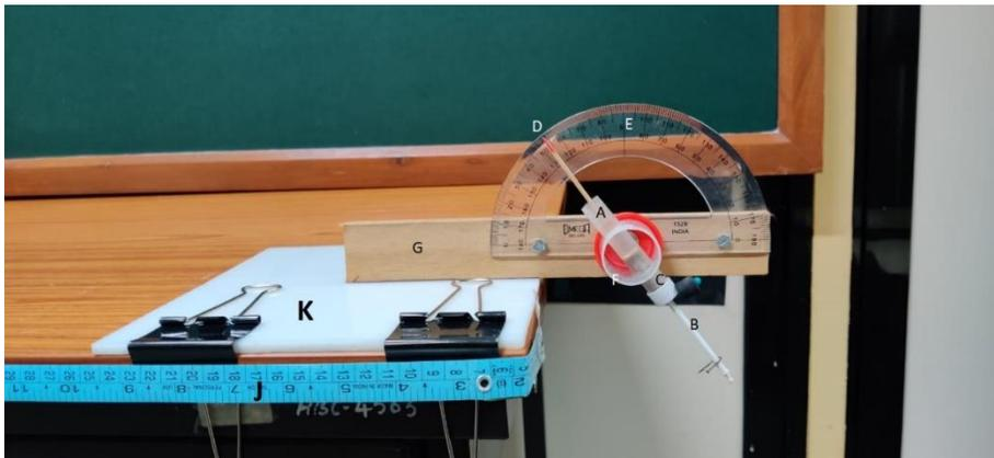
*Figure 1. The picture of launcher of the projectile attached to a table top.*
