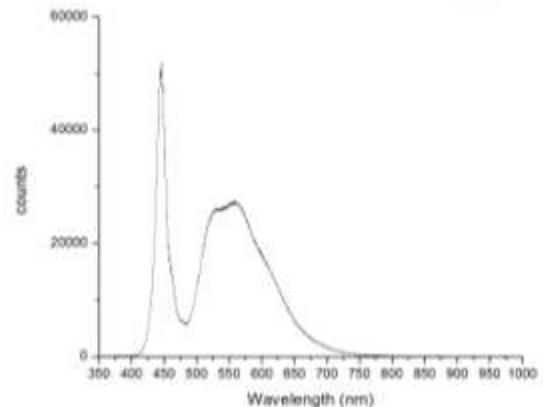
Figure 3. The spectrum of light emitted by a white LED, indicating the intensity of each of the wavelengths emitted by the white LED.
