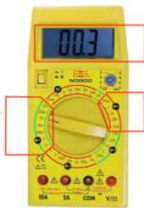
If display read  $-1$ , it implies range is insufficient. Shift the knob to higher range. Working in higher range than required will result in loss of accuracy
