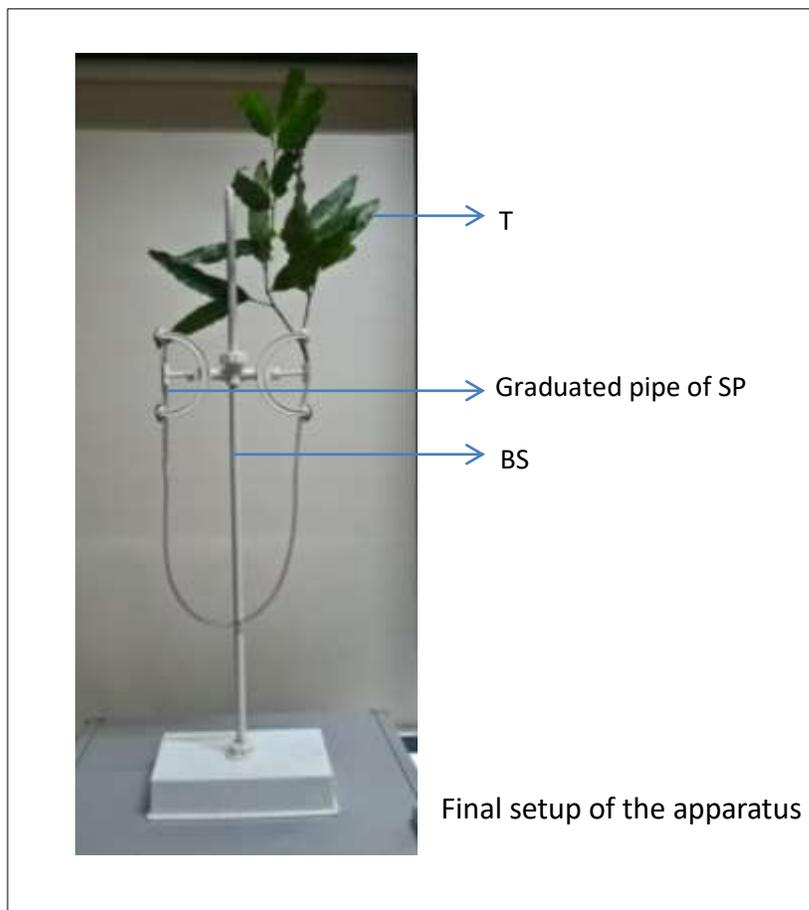
9. The water level in pipette starts decreasing gradually. Start the timer when water level reaches the first mark on pipette. Stop the timer when it reaches next mark. Record the time (t). Immediately reset the timer and start again for next reading. Take 5 consecutive readings in a same way. The distance between two marks indicates 0.1 ml volume of water. The (t) is the time taken by plant for transpiration of 0.1 ml water. Take average of all 5 readings.
